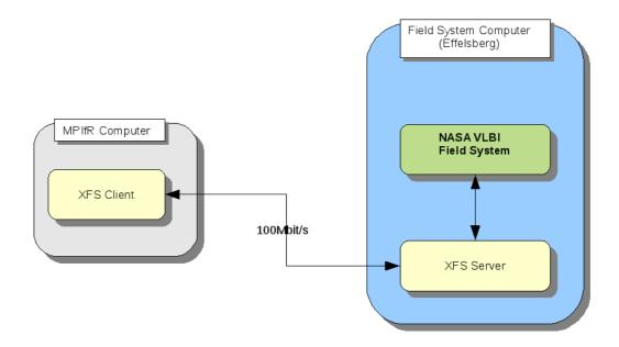
Figure 1: Sketch of the test setup. The XFS server was installed and started on the field system computer in Effelsberg. The XFS client was installed and run on a computer located at the MPIfR in Bonn.The client and server were connected over a 100 Mbit/sec line.
