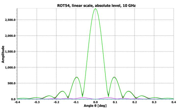
Predicted halfpower beamwidth different...: 0.08 deg (4.8') (measurement: non-linearity in scale and pointing aspects) ROT54 radio-telescope KvtK
