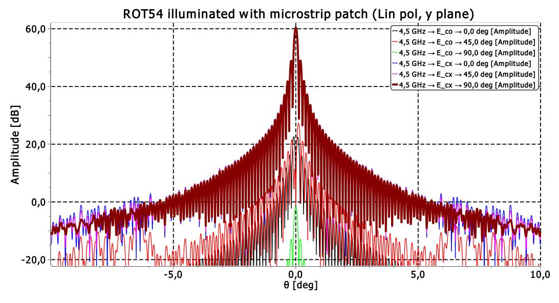
The microstrip patch is linearly polarised, assymetric feeding point, patch needs alignment !! Consequences on pointing, crosspol, spherical wave expansion patch co-aligned with ROT54 focal position
