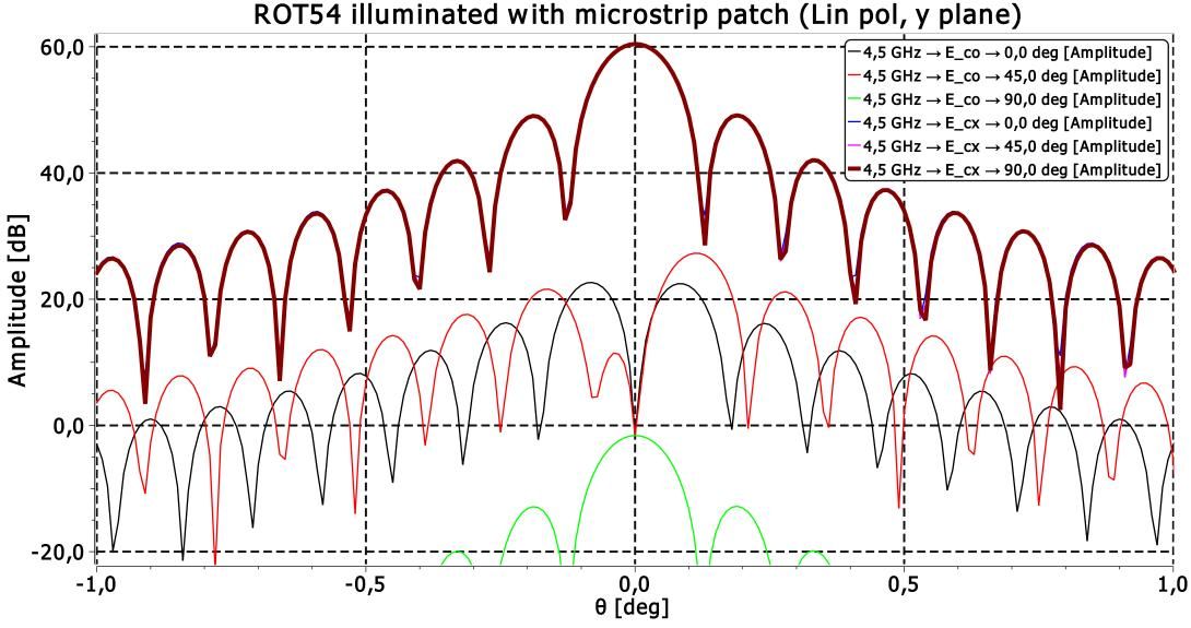
The microstrip patch is linearly polarised, assymetric feeding point, patch needs alignment !! Consequences on pointing, crosspol, spherical wave expansion patch co-aligned with ROT54 focal position
