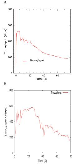
Figure 4: TCP throughput for a disk2net-net2disk e-VLBI data flow: A - Real flow, B - Simulated flow.
