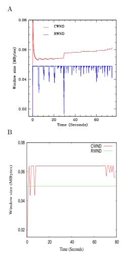
Figure 2: Congestion Window and Receive Window for a disk2net-net2disk e-VLBI data transfer (RWND steadily lower than CWND): A - Real flow, B - Simulated flow.
