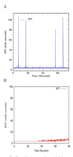
Figure 3: Round trip time for a disk2net-net2disk e-VLBI data flow between two MarkV units both in the Netherlands: A - Real flow, B - Simulated flow.
