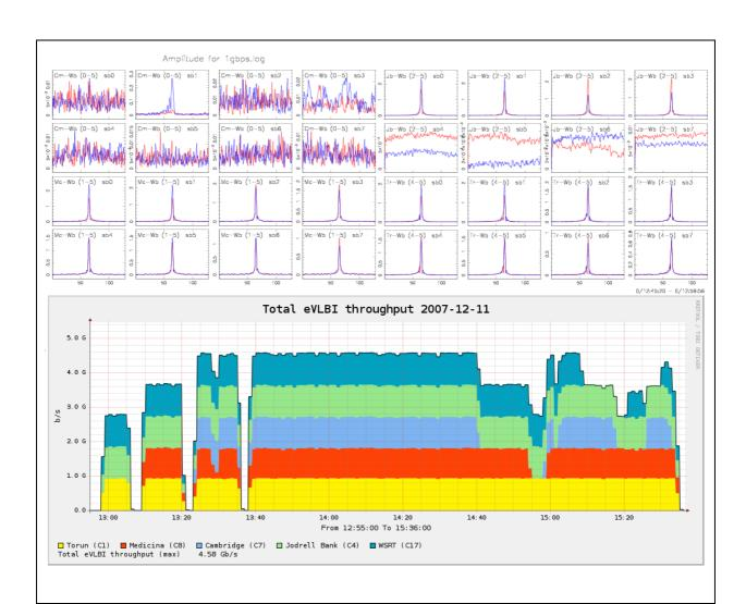
Figure: The top panel shows the fringes (some missing due to e.g. microwave link limitations). The lower panel shows the aggregate bitrate during the experiment.
