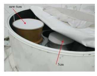
A new 6cm receiver has just been mounted on the VLBI parabolic antenna of the Medicina station, improving the sensitivity of almost a factor of two with respect to the old receiver..
