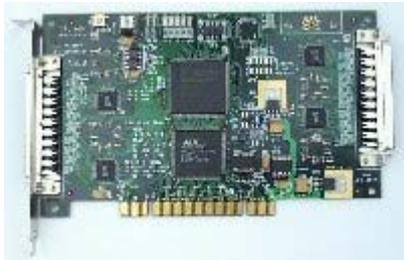
Figure 1: The Metsähovi VSI Interface Board.
